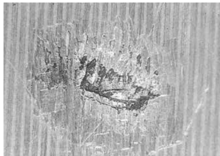
Surface fatigue on ball bearing
