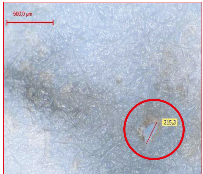
Burn hole in the filter material
