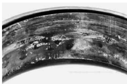
Adhesion on ball bearing
