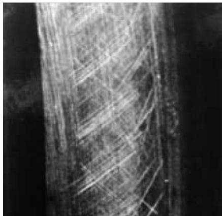
Abrasion caused by foreign bodies
