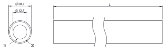
1) Fiberglass braided sleeve, 2) Red iron oxide flame protection
