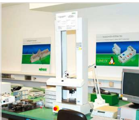
Conductor retention force testing
