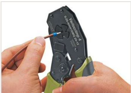
Insert ferruled conductor into crimping station.
