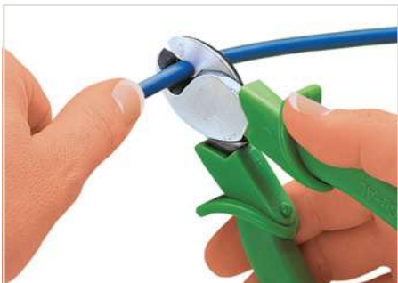
Cutting a cable.
