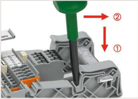
Release the fixing bracket by pushing the operating tool down ① and then forward ②.
